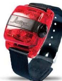
Figure 2: Actigraph for measuring physical activity (accelerometry, Source: actigraphcorp.com).
