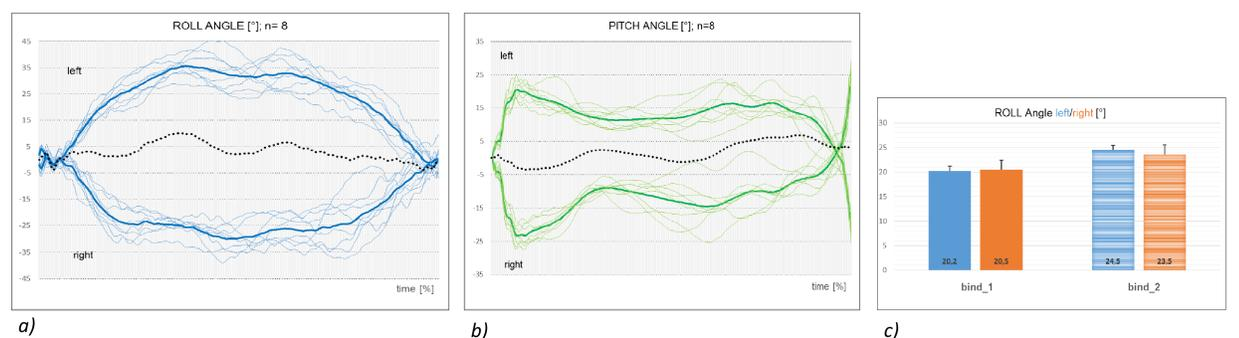
Fig. 3: roll (a) and pitch (b) angle with lateral deviation (black dotted). Roll angle in comparison to different binding systems (c).
