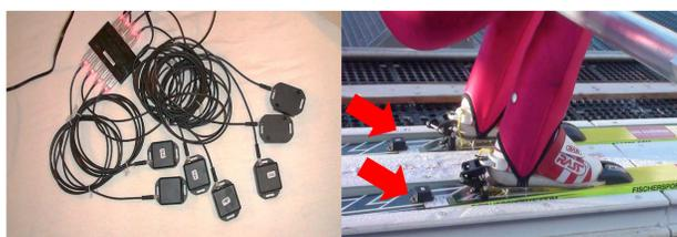
Fig. 1: Data logger connected to USB for charging (left). IMU installed on skis (right).
