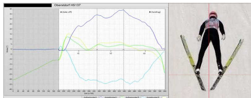
Fig. 2: L: roll (blue) and pitch (green) angle for left and right ski. R: 2d video analysis at dorsal view.
