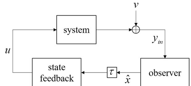
Figure 2. Optimal feedback control block diagram. We implemented the system block using (1). The output of the system block is a measurements vector which appears in Eq. 5 subject to measurement noise  $v$ . The observer block uses the measurement vector  $y$  in order to estimate the state variables of the pendulum,  $\hat{x}$ . The estimated state variables, are then delayed by  $\tau$  ms and used by the state feedback control in order to calculate the optimal control signal  $u$ .
