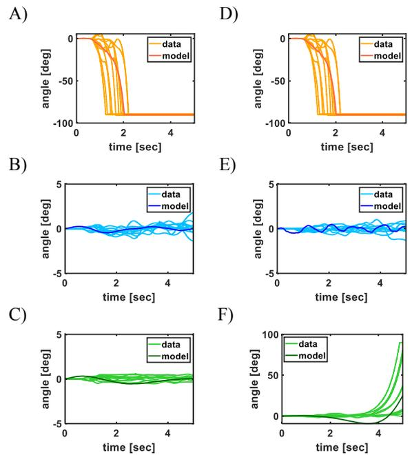
Figure 3. Examples of pendulum angle as a function of time. Examples from experiment 1 is presented in A, B, and C for conditions  $L=0.25, 1.5,$  and  $8$  respectively. In each figure we plotted 10 representative trials performed by one subject using light orange, blue and green lines. Dark orange, blue and green line represent the LQG model predictions for each condition. Examples from experiment 2 using the same notation are presented in D, E, and F.
